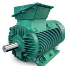
FLSES IE2 - IE3 Cast iron* IP55 Frame size from 80 to 450 mm 2, 4 and 6 poles 0.75 to 400 kW
