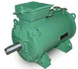
LC IE3 Liquid cooled / IP55 Frame size 315 up to 500 mm 2, 4 & 6 poles 150 up to 1500 kW
